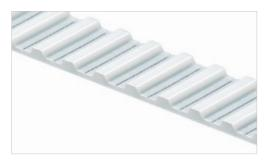
HabaSYNC® Flex timing belts offer the familiar reliability and precision of HabaSYNC®. The helically wound tensile members provide double the tensile strength of joined endless timing belts. HabaSYNC® Flex belts are ideal for conveying heavy loads; they are also used in high power transmission applications.
